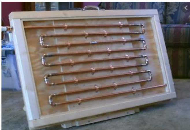
Figure 2: Cooling system using copper pipe
